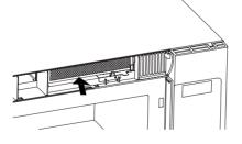
4. Lift the bottom of the charcoal filter. Slide the filter straight out.
